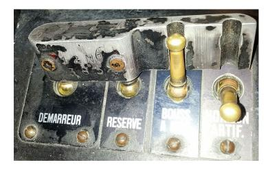
Interlocking device to prevent incompatible positions of various switches
