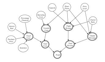
A useful starting point is to build an *influence diagram* of the relevant variables.
