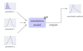
**Uncertainty analysis**: how does variability in the inputs propagate through the model to variability in the outputs?
