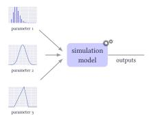
**Propagate** the input variability to the output variability by running the model a large number of times with inputs taken from the input probability distributions.
