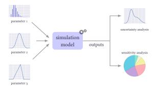
**Uncertainty analysis**: how does variability in the inputs propagate through the model to variability in the outputs?
